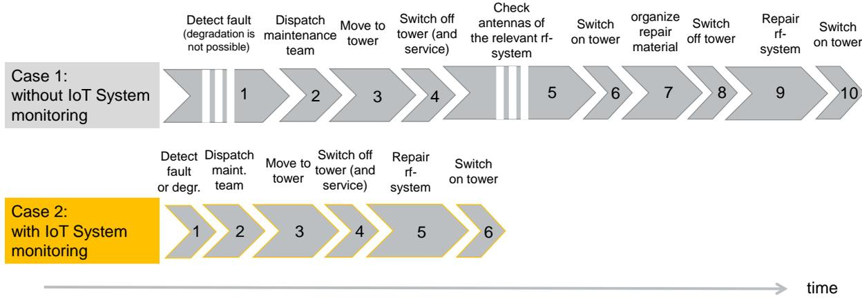
Principle illustration: time blocks are not proportional to the used time, e.g. detect fault in task No. 1 in case 1 could take very long, in case 2 it is immediate. The same issue for task No. 5 in case 1, depending on the size of the tower this task could be over proportional long.
